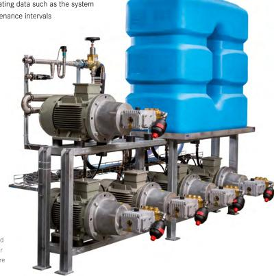
Stationary multiple-stage system 5HD 7,5/35-120, designed for five simultaneous users. This system provides every user with a water capacity of 35 l/min with an operating pressure of 120 bar.
