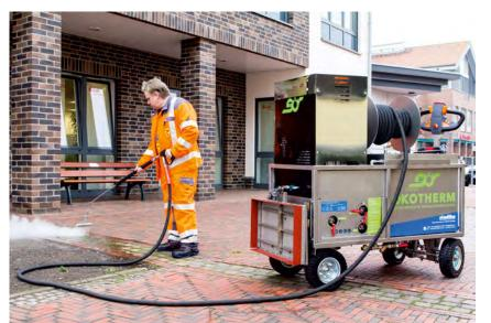
The ÖKOTHERM can be used under virtually any weather conditions. It is specially designed for communal areas in pedestrian zones, graveyards, train platforms and any public areas where weeds need to be combatted. Thanks to its compact design, the ÖKOTHERM is particularly suitable for areas which cannot be accessed by larger devices.
